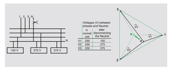
Consequences of disconnecting an evenly balanced Neutral conductor only in an installation when the single-phase loads are unevenly balanced.
